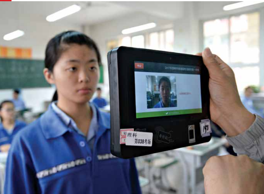
A teacher uses a machine which employs both fingerprint and facial recognition technology to check the identification of a student before a simulated college entrance exam
